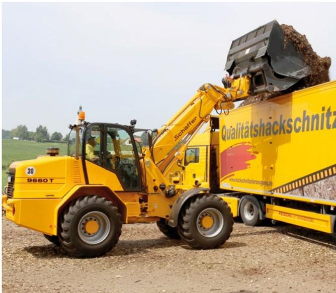
Just under twenty minutes are needed by the 9660 T and its large capacity high tilting bucket to fill the sliding floor articulated truck (bulk capacity 94 cubic metres). The lifting height with the telescopic arm **retracted** is an impressive 4.80 m.
