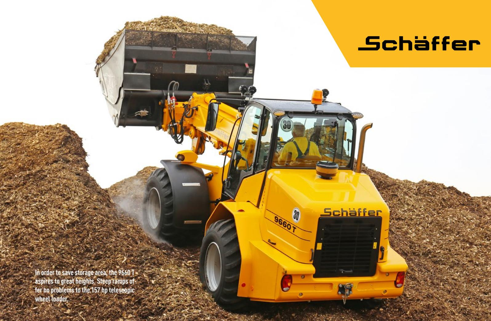
In order to save storage area, the 9660 T aspires to great heights. Steep ramps offer no problems to the 157 hp telescopic wheel loader.
