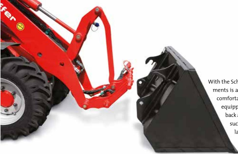
With the Schaffer headstock SWH the coupling of all attachments is a breeze. The hydraulic lock is standard and very comfortable. Genuine Schaffer attachments are also equipped with the double hook frame. Thus, the roll back and dump angle are adjusted easily. For materials such as grain a larger roll back angle is preferable. A larger dump angle is good for other material such as soil - simple, flexible, ingenious.
