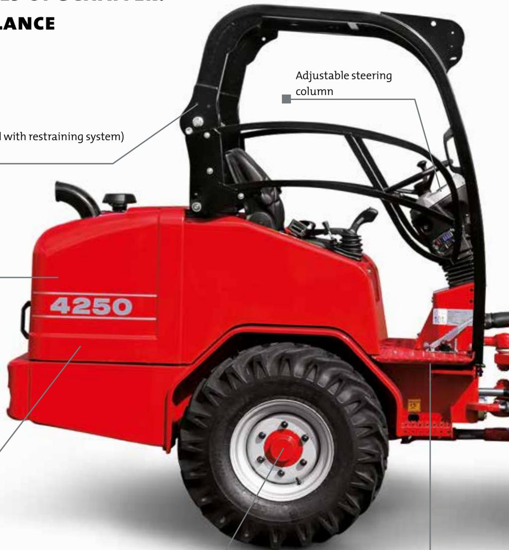
Protective roof (optional with restraining system) or cab.
