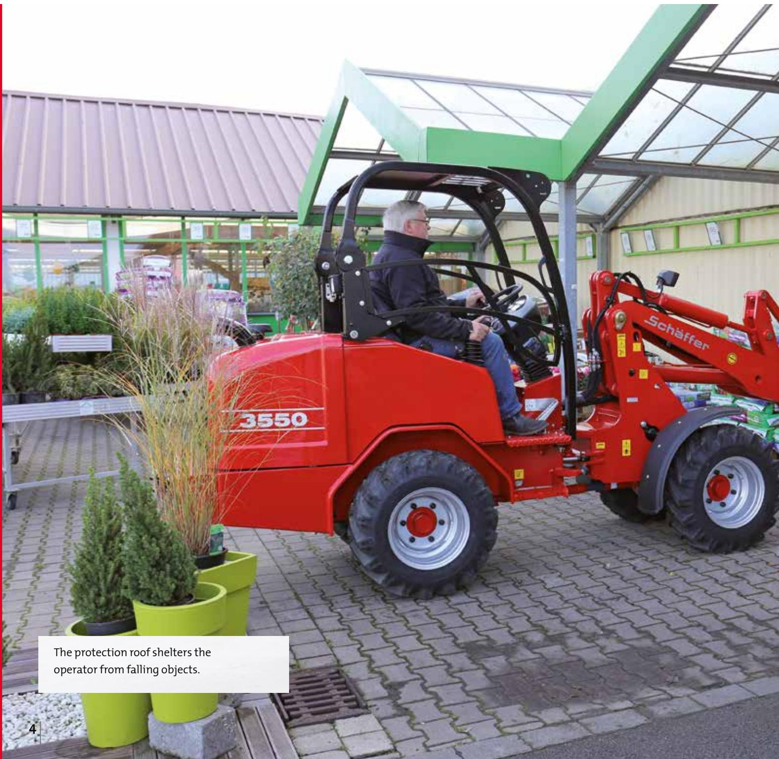
The protection roof shelters the operator from falling objects.
